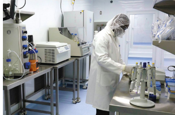
GermFree mobile cleanroom for hands-on training on cGMP fill-finish of injectables
